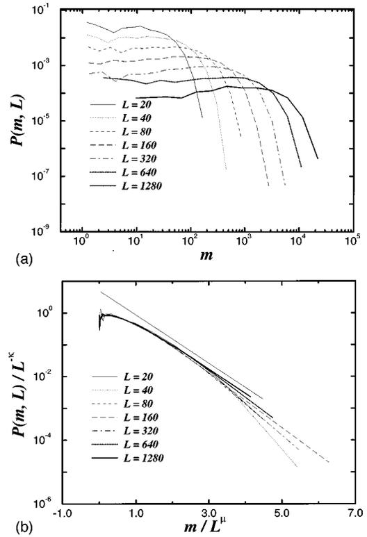
FIG. 5. (a) Log-log plot of the probability density of the sizes  $m$  of the discharge events for several system sizes. It is visually apparent that the distribution is bounded. (b) Data collapse of the curves shown in (a) according to Eq. (5) with the exponents  $\kappa = \mu \approx 1.20$ . As a visual aid, we display a line corresponding to an exponential dependence.
