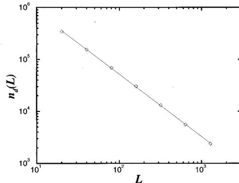
FIG. 3. The dependence of the number of discharge events  $n_d$  as a function of  $L$ . A power-law behavior, cf. Eq. (3), with  $\mu' \approx 1.20$  is obtained.
